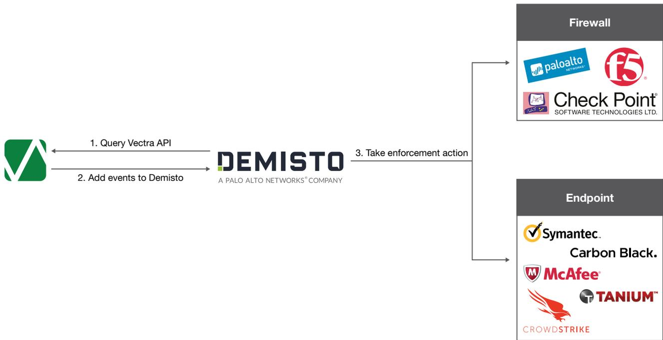
Vectra Active Enforcement for Demisto integrates with other leading security controls to stop malicious traffic or quarantine a compromised host device
